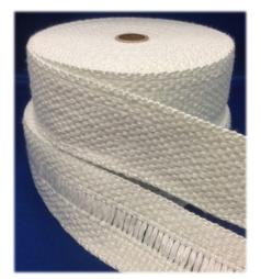
**Tetraglas**<sup>®</sup> is a woven fiberglass tape made with type E texturized yarns. Available in both a plain and drop warp weave, it has a continuous operating temperature of 1000°F/540°C and has excellent resistance to most acids, alkalis and solvents. We also offer a lighter weight **Industrial Grade** material. Both constructions can be coated with Vermiculite or PTFE.
