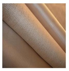
Tetraglas<sup>®</sup> 3000 silica cloth, a woven material made from amorphous silica, has a continuous operating temperature of 1800°F/980°C. It has excellent resistance to most acids, alkalis, solvents, and is an excellent alternative to Refractory Ceramic Fiber (RCF).
