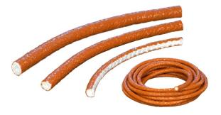
Silco Rope<sup>®</sup> is designed to provide a seal in environments that are exposed to the hazards of high heat and occasional flame. It protects continuously to 500°F/260°C and will withstand a molten splash at 2200°F/1200°C. Made of knitted type E fiberglass rope, it is then coated with a high grade silicone rubber.
