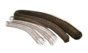
Our knitted mesh cables and tapes are used in a variety of products and applications. Our cables provide compressive strength as the fill in the bulb or tail of high temperature industrial and commercial gaskets. Our tapes are widely used to provide EMI/RFI shielding for electronic enclosures, and in combination with silicone gels to offer an additional environmental seal.
