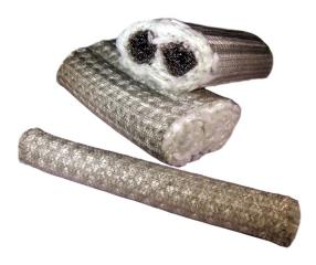
Our Custom Seals are constructed of high quality Type E glass yarns with a knitted 304 stainless steel wire jacket for superior abrasion resistance. The high temperature glass yarns will not burn and provide continuous exposure to temperatures of 1000°F/540°C. Moreover, the compressive strength of the knitted fiberglass rope preserves the shape of the Seal after repeated use.
