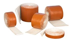
Silco Tape<sup>®</sup> is designed to protect hoses, wires and cables from the hazards of high heat and occasional flame. It protects continuously to 500°F/ 260°C and will withstand a molten splash at 2200°F/1200°C. Made of knitted fiberglass yarns in a flexible substrate, it is then coated with a high grade silicone rubber.
