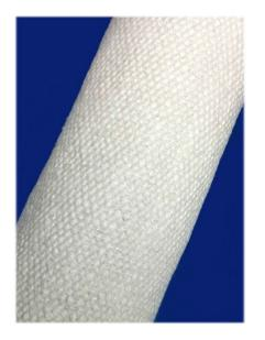
Our ceramic cloth is a woven material made from alumina-silica ceramic fiber and has a continuous operating temperature of 2300°F/1260°C. It has excellent chemical stability and strong resistance to thermal shock and corrosion attack.
