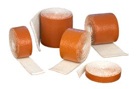
Silco Tape® is designed to protect hoses, wires and cables from the hazards of high heat and occasional flame. It protects continuously to 500°F/ 260°C and will withstand a molten splash at 2200°F/1200°C. Made of knitted fiberglass yarns in a flexible substrate, it is then coated with a high grade silicone rubber.
