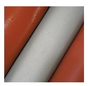
Tetraglas® and Tetraglas 3000® woven cloths with high grade silicone rubber are a versatile solution to high temperature protection needs. With a continuous operating temperature up to 500°F /260°C, our silicone coated cloths will withstand a molten splash at 2200°F/1200°C and are resistant to hydraulic fluids, lubricating oils, and fuels.
