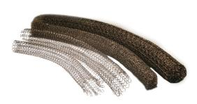
Our knitted mesh cables and tapes are used in a variety of products and applications. Our cables provide compressive strength as the fill in the bulb or tail of high temperature industrial and commercial gaskets. Our tapes are widely used to provide EMI/RFI shielding for electronic enclosures, and in combination with silicone gels to offer an additional environmental seal.
