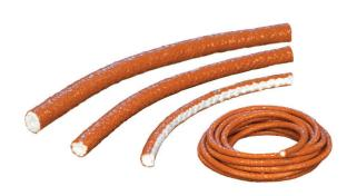
Silco Rope® is designed to provide a seal in environments that are exposed to the hazards of high heat and occasional flame. It protects continuously to 500°F/260°C and will withstand a molten splash at 2200°F/1200°C. Made of knitted type E fiberglass rope, it is then coated with a high grade silicone rubber.
