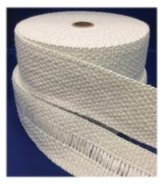
**Tetraglas**<sup>®</sup> is a woven fiberglass tape made with type E texturized yarns. Available in both a plain and drop warp weave, it has a continuous operating temperature of 1000°F/540°C and has excellent resistance to most acids, alkalis and solvents. We also offer a lighter weight **Industrial Grade** material. Both constructions can be coated with Vermiculite or PTFE.
