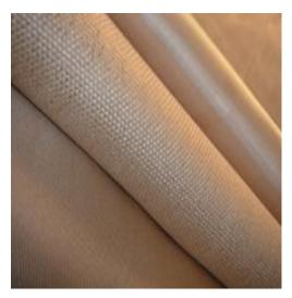
Tetraglas<sup>®</sup> 3000 silica cloth, a woven material made from amorphous silica, has a continuous operating temperature of 1800°F/980°C. It has excellent resistance to most acids, alkalis, solvents, and is an excellent alternative to Refractory Ceramic Fiber (RCF).
