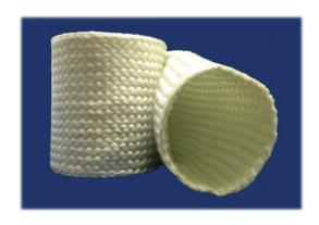
**Tetraglas® Sleeves** are braided fiberglass sleeve made with type E texturized yarns. It is available with either a 1/16" (1.6mm) or 1/8" (3.2mm) thick wall and offers a continuous operating temperature of 1000°F/540°C. It provides excellent resistance to most acids, alkalis and solvents. Vermiculite, PTFE, and graphite coatings can be added to this product to add to its versatility.
