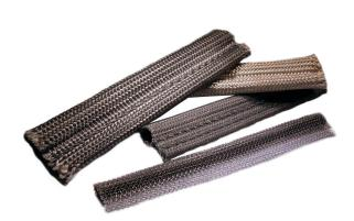
Our tadpole gaskets are designed to provide a high temperature thermal seal in industrial, laboratory, commercial, and residential ovens and dryers with a maximum continuous operating temperature of 1000°F/540°C. Constructed with type E fiberglass, the bulb may be filled with various constructions of either fiberglass or stainless steel in order to achieve the proper design compression.
