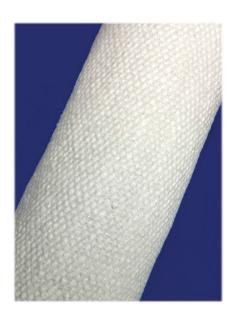
Our ceramic cloth is a woven material made from alumina-silica ceramic fiber and has a continuous operating temperature of 2300°F/1260°C. It has excellent chemical stability and strong resistance to thermal shock and corrosion attack.
