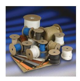
**Tetraglas**<sup>®</sup> round knitted, twisted, and square braided ropes are constructed of high quality type E fiberglass yarns, which offer a continuous service temperature up to 1000°F/540°C. This material resists most acids and alkalis; is unaffected by most bleaches and solvents; and is highly flexible and conformable. Knitted Tetraglas<sup>®</sup> rope is offered in two styles: soft and dense.
