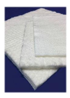
We offer three types of blanket materials that provide thermal insulation and protection at high temperatures while offering excellent resistance to most acids, alkalis and solvents. These blankets are made from fibers that are mechanically needled together without chemical binders.
